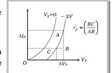
It is expressed in kilo ohms ( $K\Omega$ ). Typically, it ranges from about 8  $K\Omega$  to 40  $K\Omega$ . The  $r_p$  can be determined from plate characteristics. It represents the reciprocal of the slope of the plate characteristic curve.
